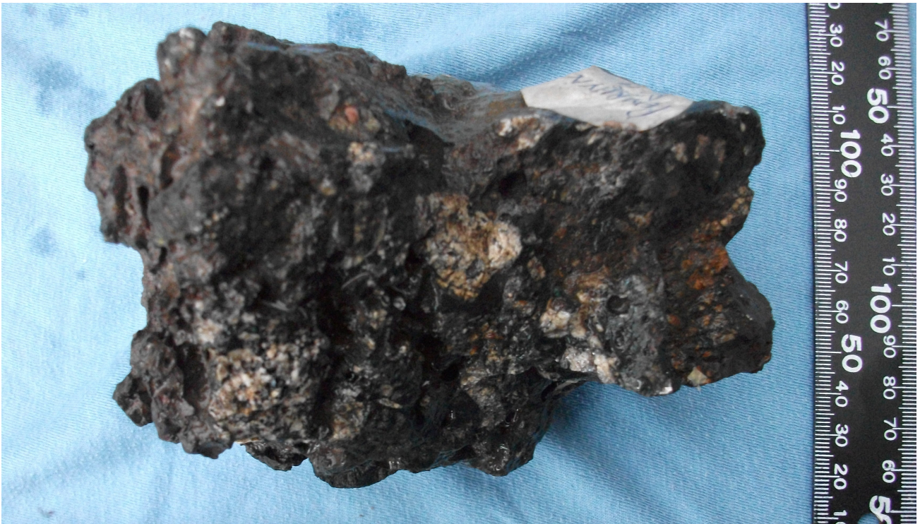
Type 2 Slag, Port Penrhyn, showing numerous 'frothy' holes.
